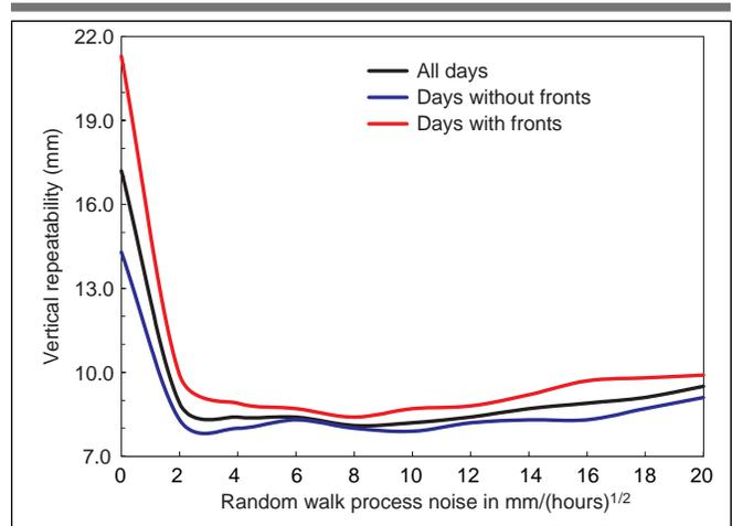
Figure 7. Repeatability as a function of random walk process noise and the passage of weather fronts at Herstmonceux. Days affected by weather fronts are more sensitive to the
