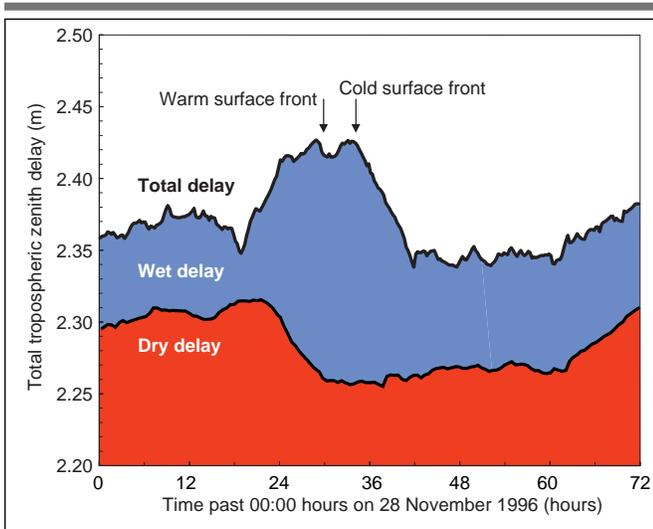
Figure 5. Total, dry, and wet delays as fronts pass
