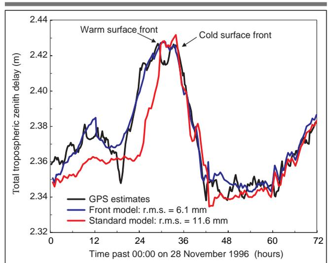
Figure 4. GPS-estimated and model-predicted total zenith path delay at Herstmonceux, 28 to 30 November 1996
