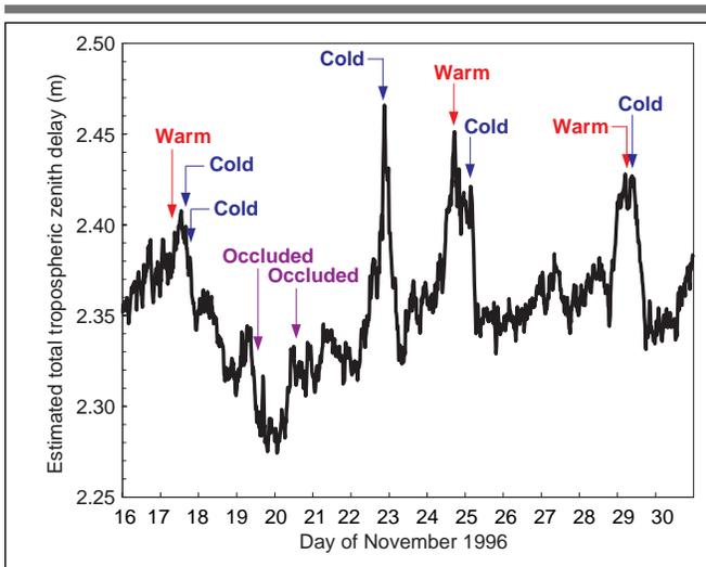
Figure 3. Tropospheric zenith delay at Herstmonceux, southern England, during a fortnight in November 1996. The passages of the surface fronts are marked as warm, cold, or occluded.
