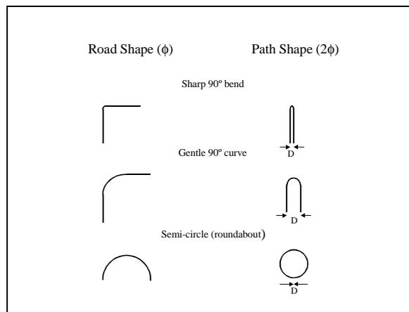
**Figure 8.** Basic road shapes can be transformed into path shapes with twice the curvature, which can then be interpreted in terms of favorable geometry (MDOP).
