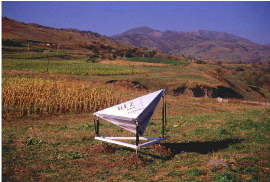
Fig. 5.3.2.6: Corner Reflector in Southern Kyrgyzstan supporting interferometric analysis of ERS-1/2 SAR data.
