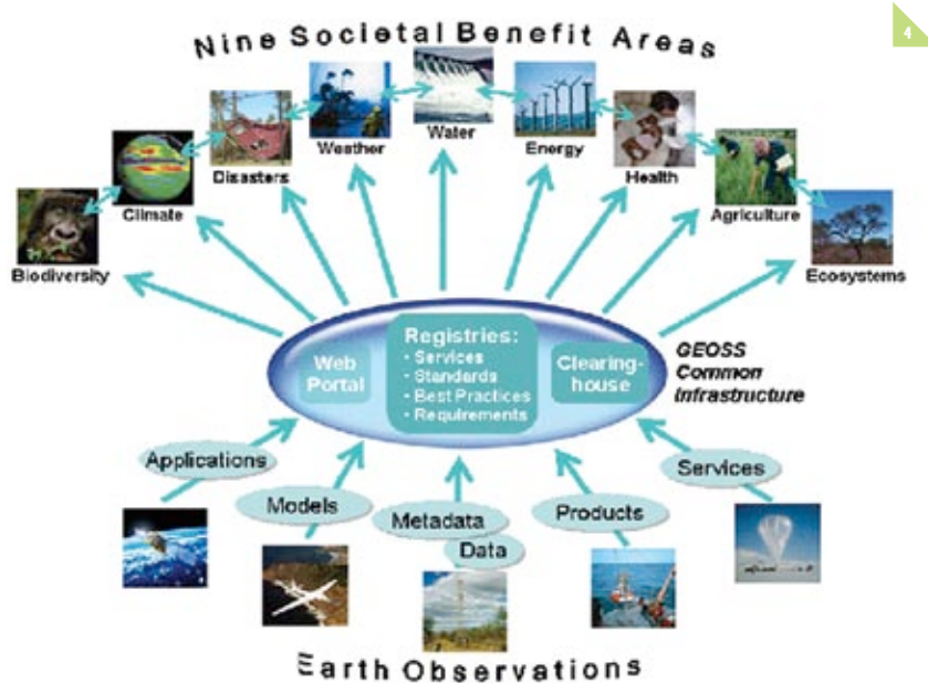
◀ FIGURE 3. The GEO Portal giving access to metadata for a global network of services, datasets, and products.
