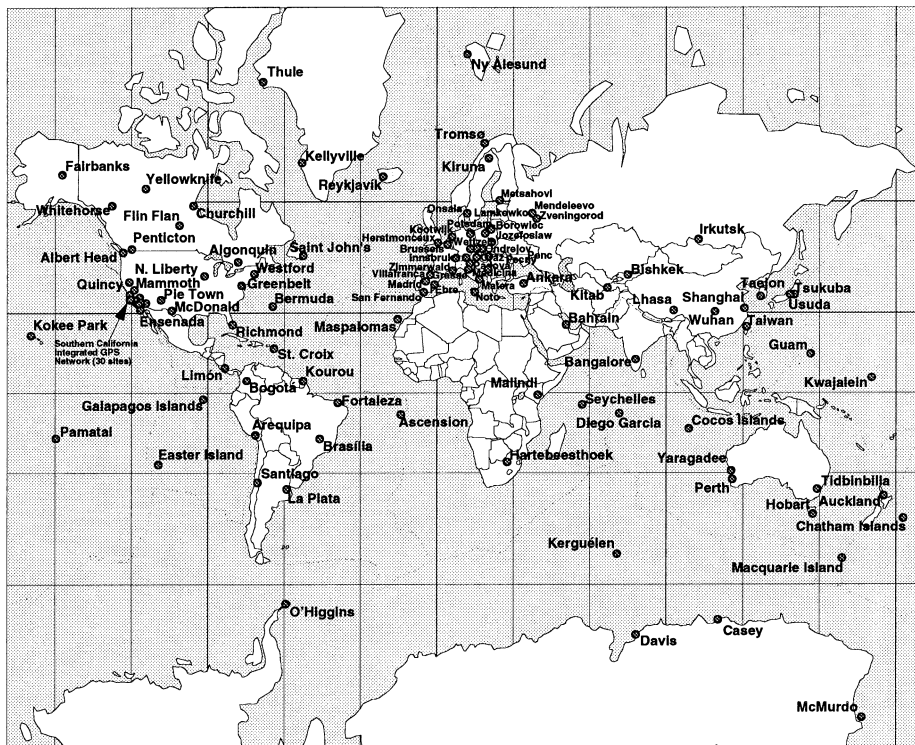
Fig. 3. Current global network of permanent GPS stations supporting the IGS.
