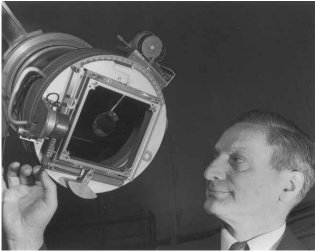
Figure 3. Dr W Markowitz with the dual-rate moon camera which he designed in 1951 for the purpose of timing the occultation of stars by the moon and hence relating UT2 to ET (photograph reproduced by kind permission of the US Naval Observatory, James M Gilliss Library Archives).
