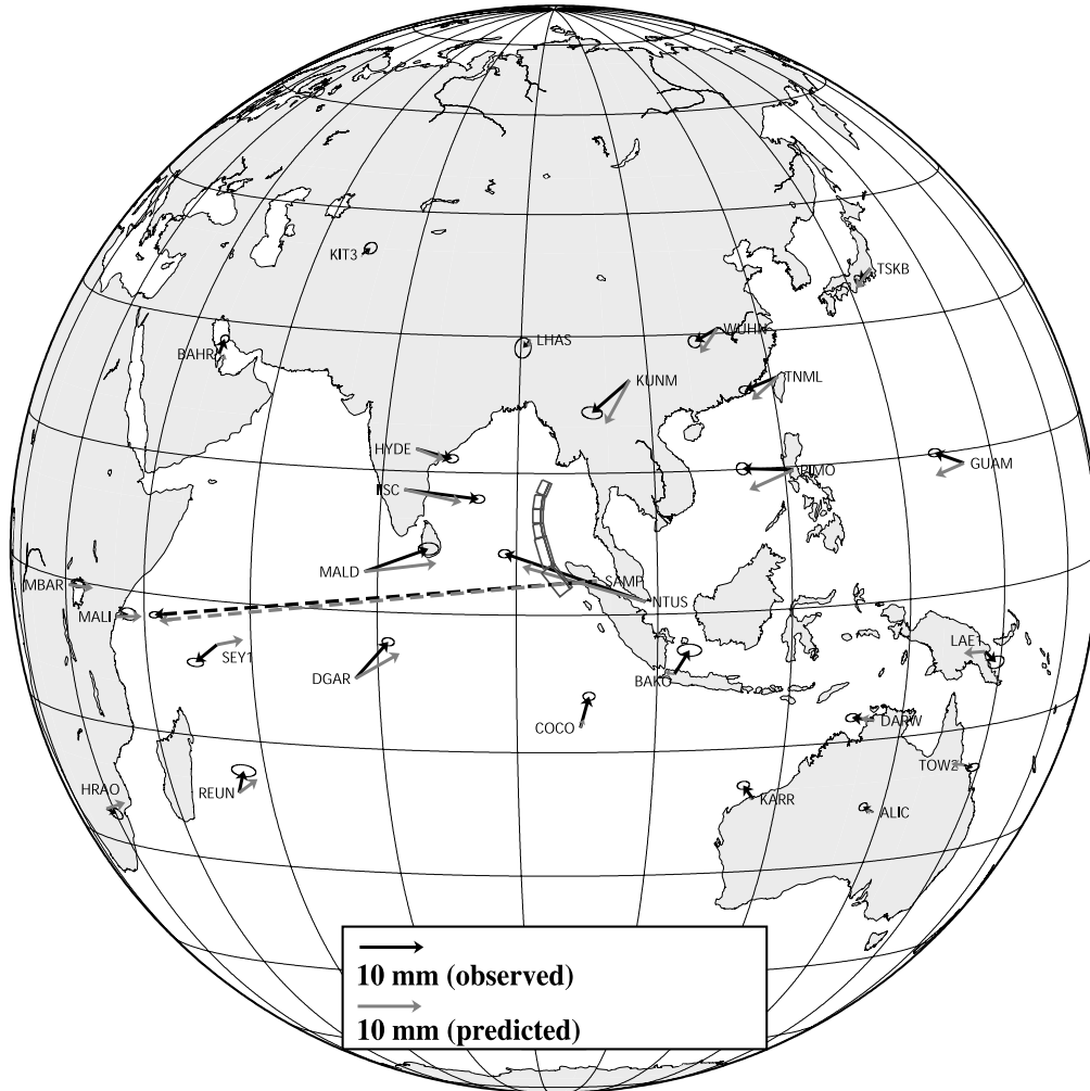
Fig. 4. Observed coseismic displacements from this study and predicted displacements from model C. Uncertainties in observed vectors are shown as 68% confidence ellipses. Rupture segments are shown in dark gray. The dashed displacements for station SAMP are plotted at half the scale as the other vectors.
